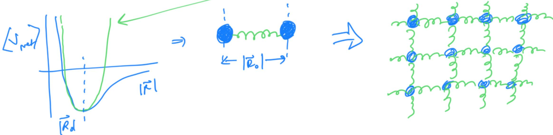
Classical estimate of  $\langle E \rangle = N [\langle KE \rangle + \langle PE \rangle] = N \left[ \frac{3}{2} k_B T + \frac{3}{2} k_B T \right]$
